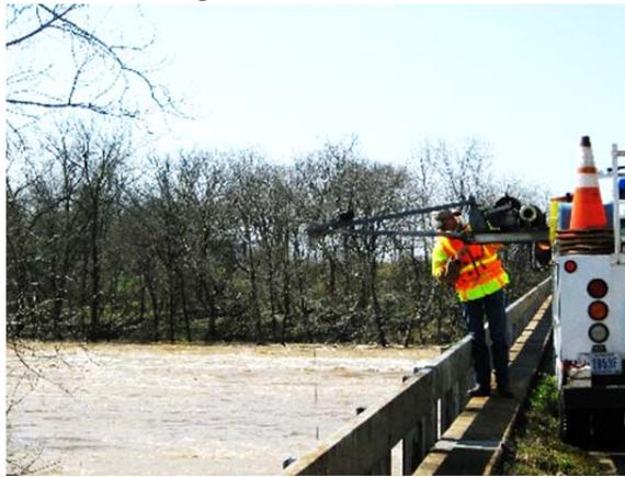
Measuring streamflow during a flood on the Illinois River.
