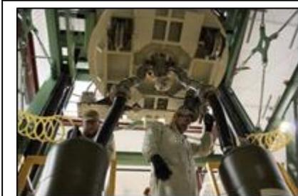
Explosives workers monitor the transfer of explosives into the body of a BLU-109 C/B penetrator bomb during first article acceptance testing at McAlester Army Ammunition Plant, Okla., Oct. 1, 2014. The 600-gallon mixing bowl rolls on a track to the back of the new B-Line facility where it is then elevated for the mix to be transferred into the bomb body that is secured below. (U.S. Army photo by Kevin Jackson, MCAAP Public Affairs)
