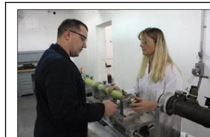
An explosives operator gets hands-on training with the disassembly of a Stinger missile from an electronic integration system mechanic journeyman in the Precision Munitions Division, Ammunition Operations Directorate at McAlester Army Ammunition Plant, Okla. MCAAP began upgrading more than 2,000 Stinger missiles in October 2014 to return them to the Department of Defense inventory. (U.S. Army photo by Kevin Jackson, MCAAP Public Affairs)
